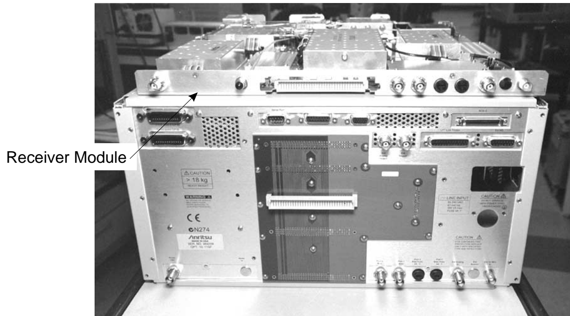
Figure 6-5. Rear Panel Showing Receiver Module Placed for Easy Access
