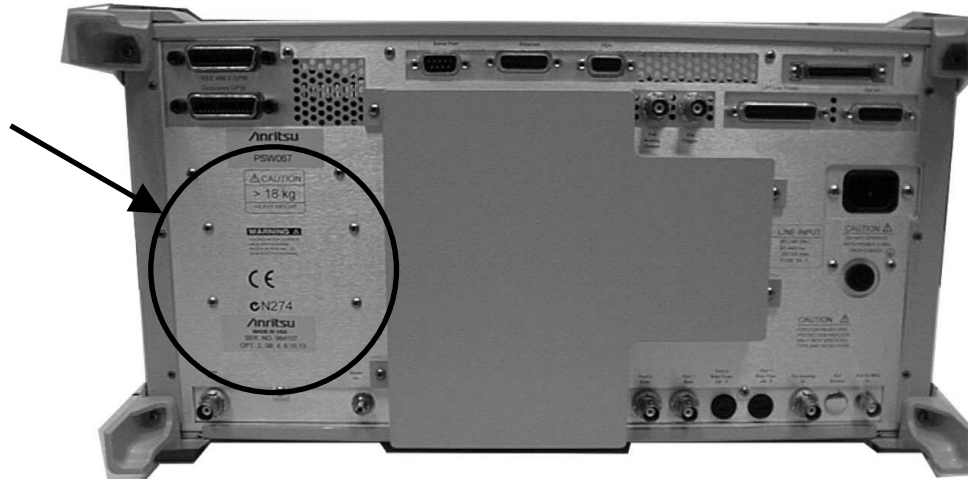
Figure 7-13. Option and Source Module Mounting Screws
